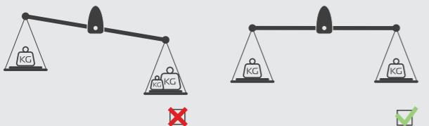
The center of gravity of the load should always be in the middle of the wheel axle.
