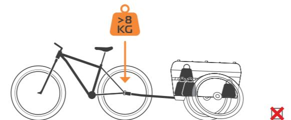
An **excessive** load leads to a poor driving behavior.
