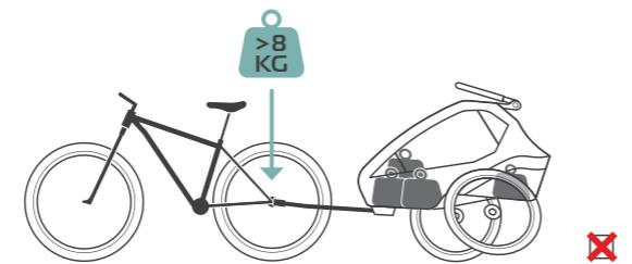
An **excessive** load leads to a poor driving behavior.
