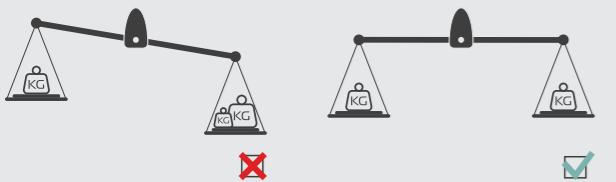
The center of gravity of the load should always be in the middle of the wheel axle.
