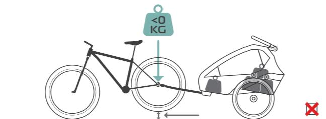
A **too low** tow bar load can push the bike upwards.
