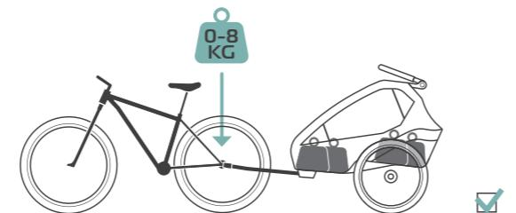
An **optimal** tow bar load ensures a safe driving behavior.
